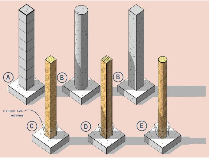
Where termites are known to exist, exterior wood columns must be pressure treated with a chemical toxic to termites and supported on a non-cellulosic base that extends to 150mm (6") above grade and is located at least 50mm (2") from the exterior wall of an adjacent building. **Separate wood columns from concrete at their base with 0.5mm polyethylene as shown.**
