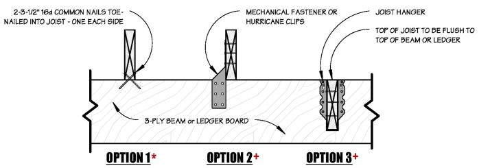
\* OPTION 1 SHALL ONLY BE USED IF DECK IS ATTACHED TO HOUSE + SEE MANUFACTURERS RECOMMENDATIONS FOR ADDITIONAL REQUIREMENTS
