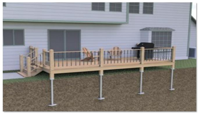
Cross-Section example showing helical pile foundation
