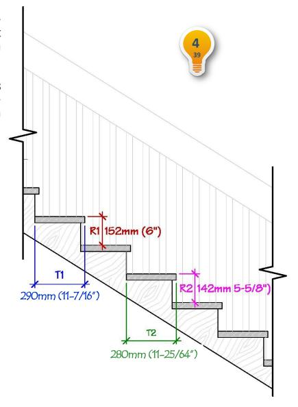
The maximum tolerance between the deepest *Tread* and the shallowest *Tread* must **not** be more than 10mm (3/8")
