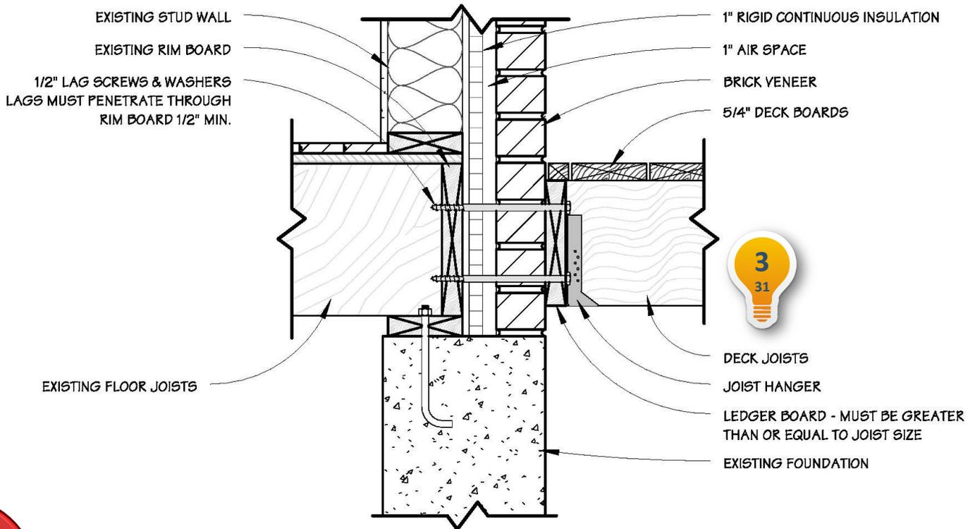
**LEDGER BOARD CONNECTIONS TO WALLS WITH NON-STRUCTURAL BRICK VENEER MUST BE REVIEWED AND SEALED BY A LICENSED STRUCTURAL ENGINEER.**
