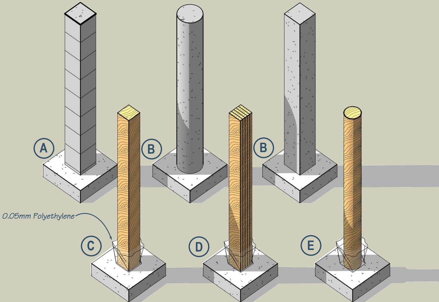
Where termites are known to exist, exterior wood columns must be pressure treated with a chemical toxic to termites and supported on a non-cellulosic base that extends to 150mm (6") above grade and is located at least 50mm (2") from the exterior wall of an adjacent building. **Separate wood columns from concrete at their base with 0.05mm polyethylene as shown.**
