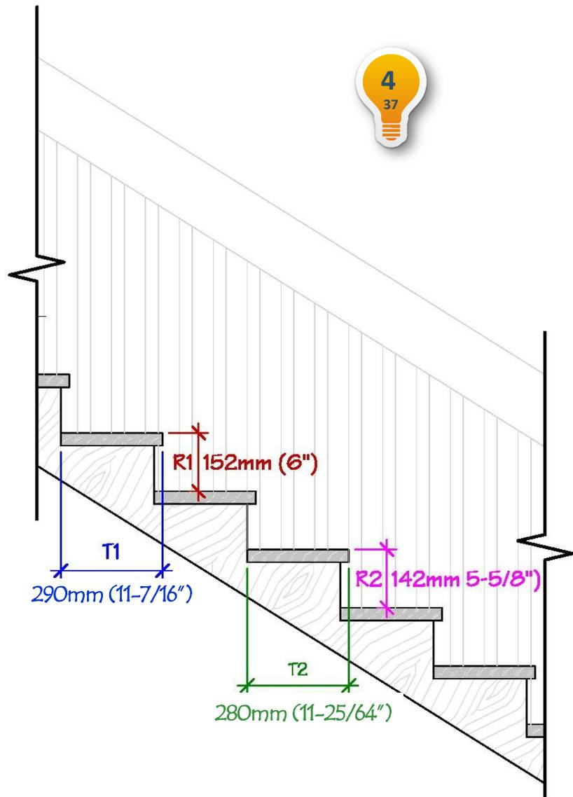
The maximum tolerance between the deepest *Tread* and the shallowest *Tread* must **not** be more than 10mm (3/8")
