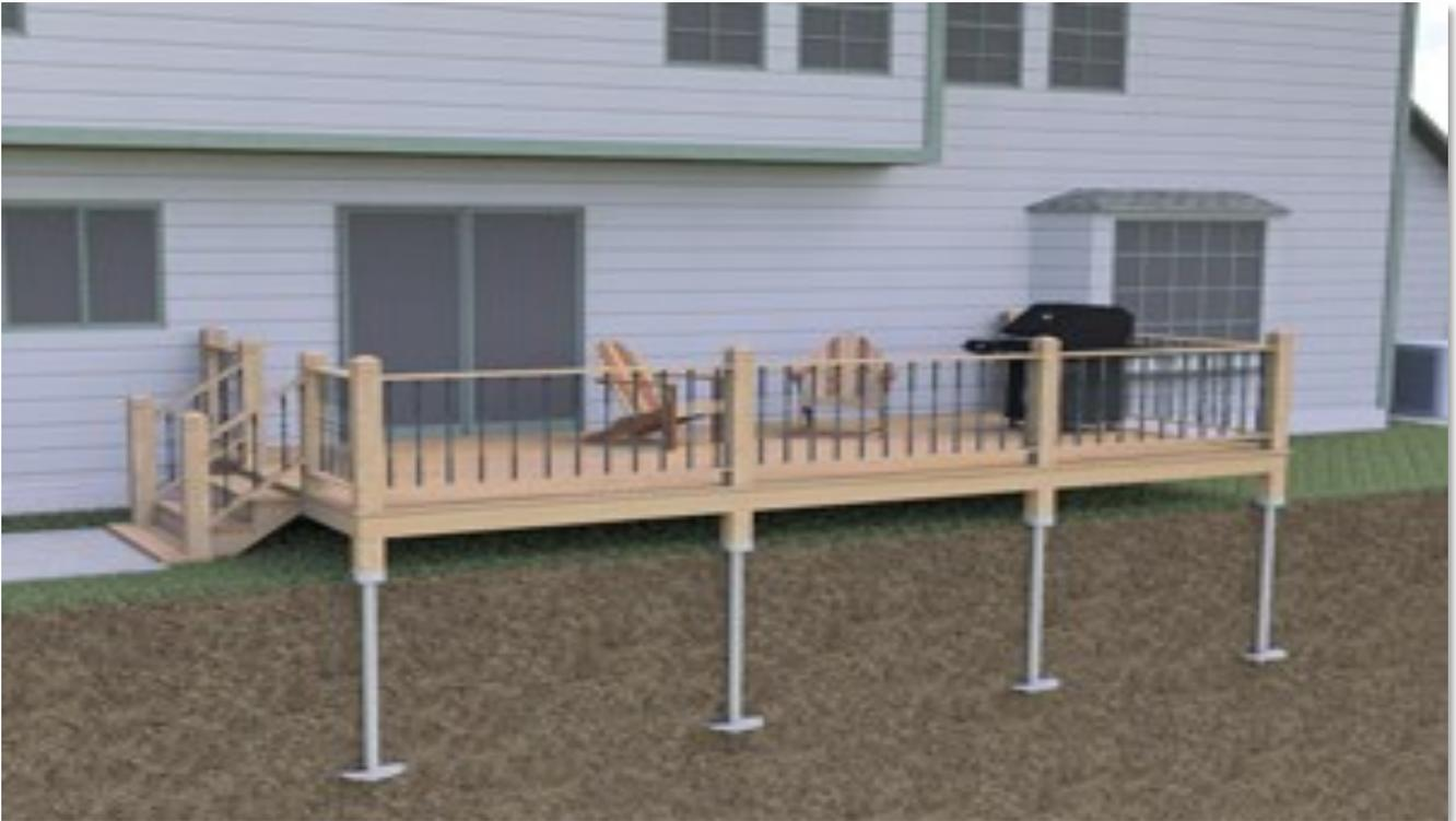
Cross-Section example showing helical pile foundation
