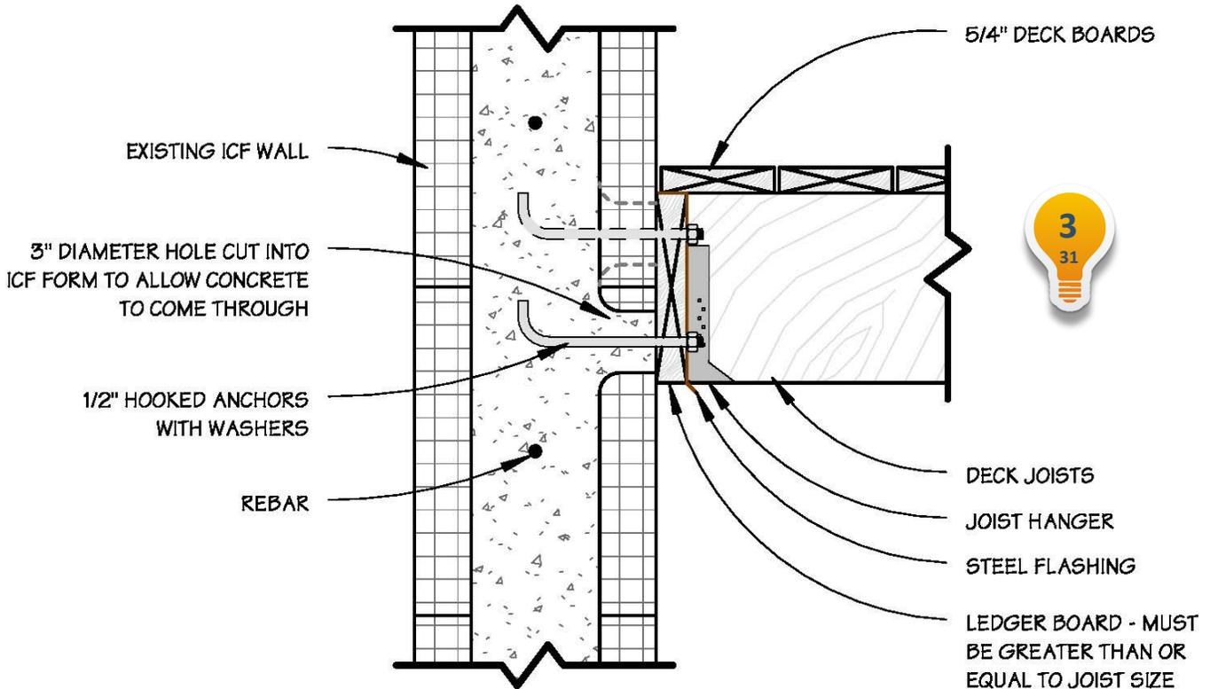
\* DECKS ADDED TO ICF BUILDINGS POST CONSTRUCTION MUST HAVE LEDGER BOARD CONNECTION ENGINEERED.
