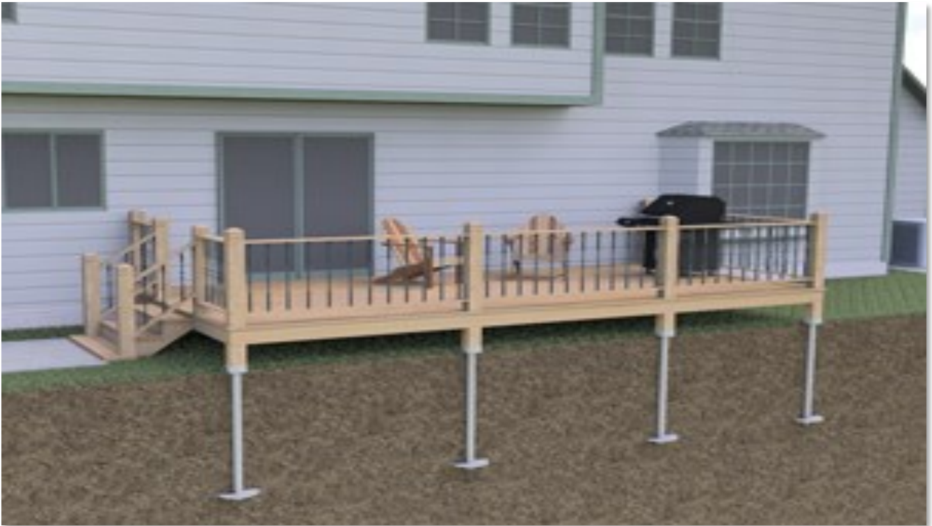
Cross-Section example showing helical pile foundation
